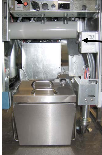
Melting unit power switch
